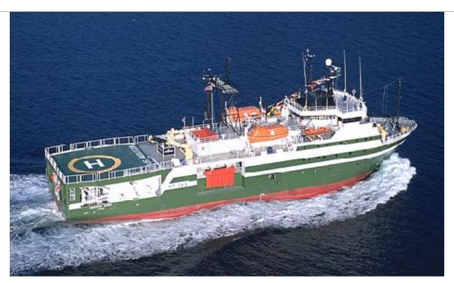
The vessel is designed by Ulstein International AS in close cooperation with Western Geophysical, and is excuted by Ulstein Verft AS as yard no. 234. The UT 743 design is developed in accordance with the demanding requirements for silent operation at high capacity production. The vessel features a compact and efficient layout, providing a comprehensive arrangement of mechanical and electronic seismic outfitting, and a highly flexible, redundant and powerful propulsion and machinery package.
